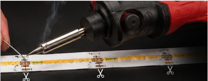
Fine point on the pad - solder fed from the side - cut marks visible on the strip
